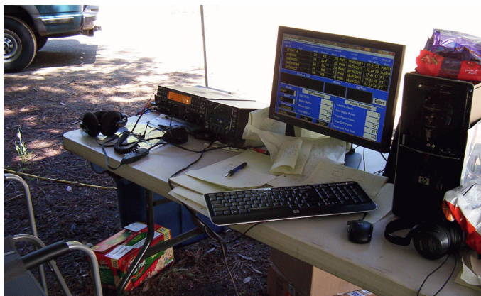
The phone station. It's hard to see here, but the rig is a K3 with the companion "waterfall" 30 kHz wide frequency spectrum analyzer. Once you got used to how a SSB station appears on the analyzer, it became a snap to see stations within 15 kHz of your frequency and jump on over to them.
